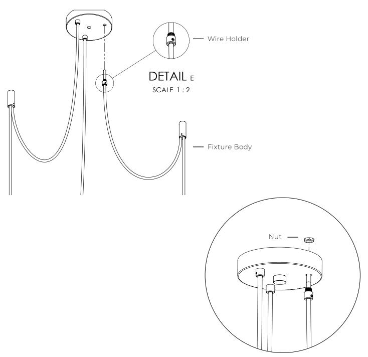
4. Person 1 lifts fixture by canopy up to the junction box. Person 2 connects fixture ground wire to ceiling ground wire, and +/- fixture wires to the +/- ceiling wires. Feed the nipple through the canopy until it is exposed at the bottom, and attach the bottom cap to the nipple and tighten until it is flush with the canopy
