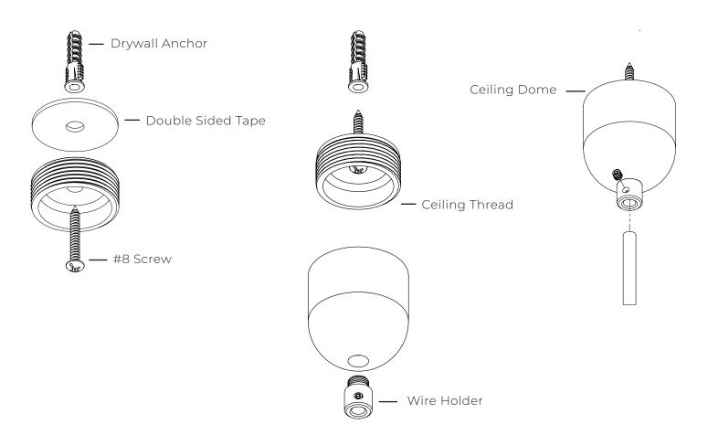
7. Once the fixture body and ceiling dome installation is complete, it should match the image below. Repeat the process for the remaining fixture body assemblies.
