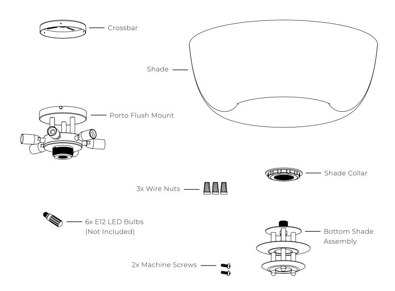
1. Mount the crossbar to the j-box using the 2x machine screws, making sure to pull the ceiling wires through to be accessible.
